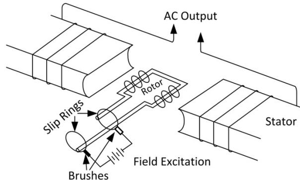
**Fig. 8 - Illustrative diagram of a synchronous generator.**
