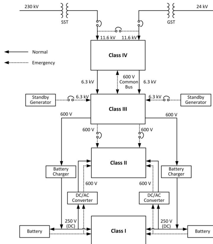
**Fig. 4 - Interconnections of different classes of power supplies.**
