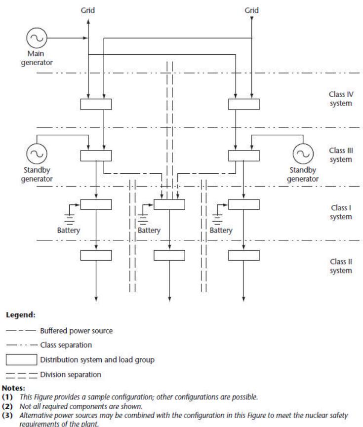
**Fig. 1 - Relationships between the station power and the power grid [1].**
