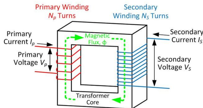
**Fig. 12 - Basic operating principle of a transformer.**
