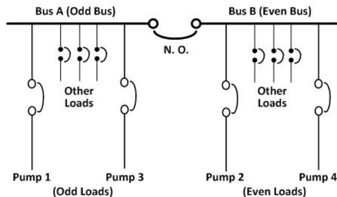
**Fig. 5 - Dual-bus configuration for power distribution systems.**
