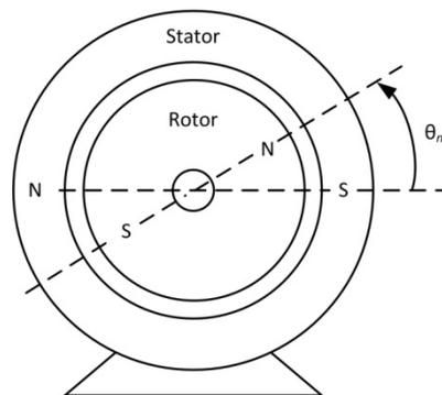
**Fig. 9 - A two-pole (one pole pair) synchronous generator.**
