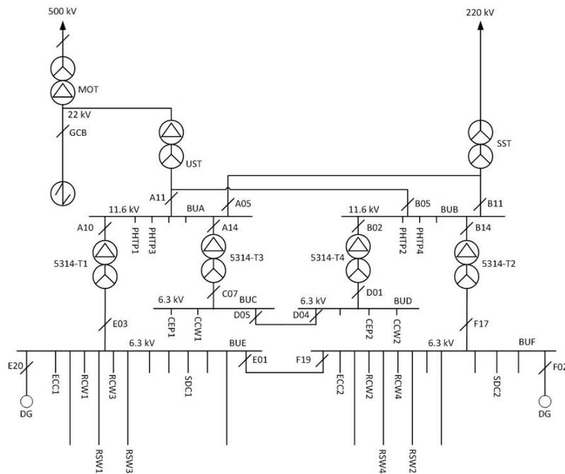
**Fig. 6 - Load distribution on the Class IV bus in a CANDU plant.**
