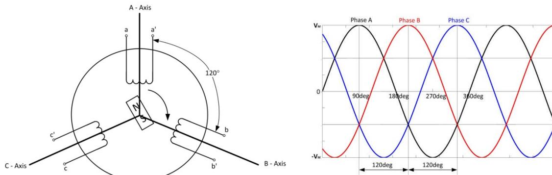
**Fig. 10 – Three-phase synchronous generator.**
