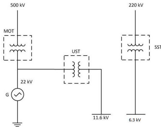
**Fig. 2 - Voltage levels within a CANDU plant.**
