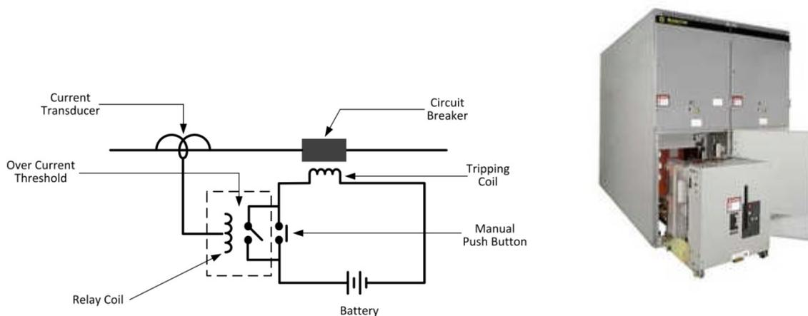
**Fig. 15 - An over-current protection circuit breaker.**
